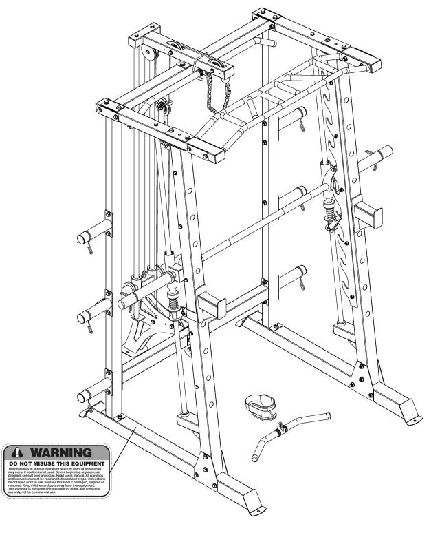
The warning labels shown here have been placed on the Cross Brace, Rear Stabilizer, and Upper Frame. If the labels are missing or illegible, please call customer service at 1-800-999-8899 for replacements. Apply the labels in the location shown.
